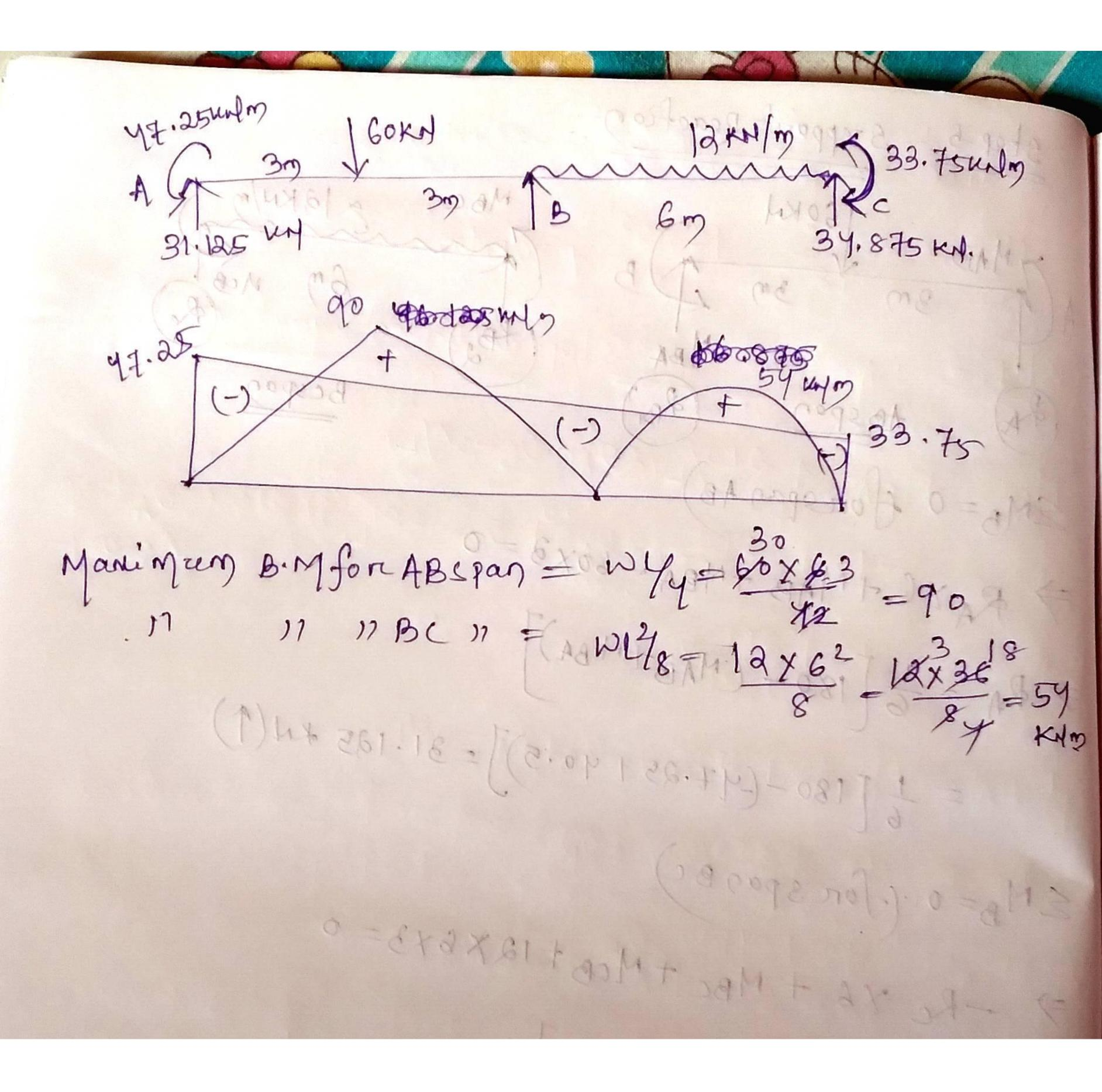
DRAW SFDagd BMD Slope deflection method. (1) finedend Moment MFAB = - WLY12 = -20.833 KND MFBA = +N4/12 = 10 x 58/12 = 20,833 KND. MFBC = - waby = - 30x 1x22 = -13.33 KNm MFCB= +Wa26/12= 30+ x12x2 -Apply slope défuetion equation foreachepan MAB = MFAB + QEITL (201+03-341)° = -20.833+ AEI/5 (0B) = -20.833+3-EIOB MBA = MFBA + RETL (208+24-3ATL) [= 20.833 + 4EI DB]. - (2) MBC = MFBC+ 2ETL (20 Bt DE-3AM). = -13.33 + 2ET/3 (20B) = [-13.33+ \frac{4}{3} Eros MCB = MFCB+ RET/L (20c+ OB-34)L
