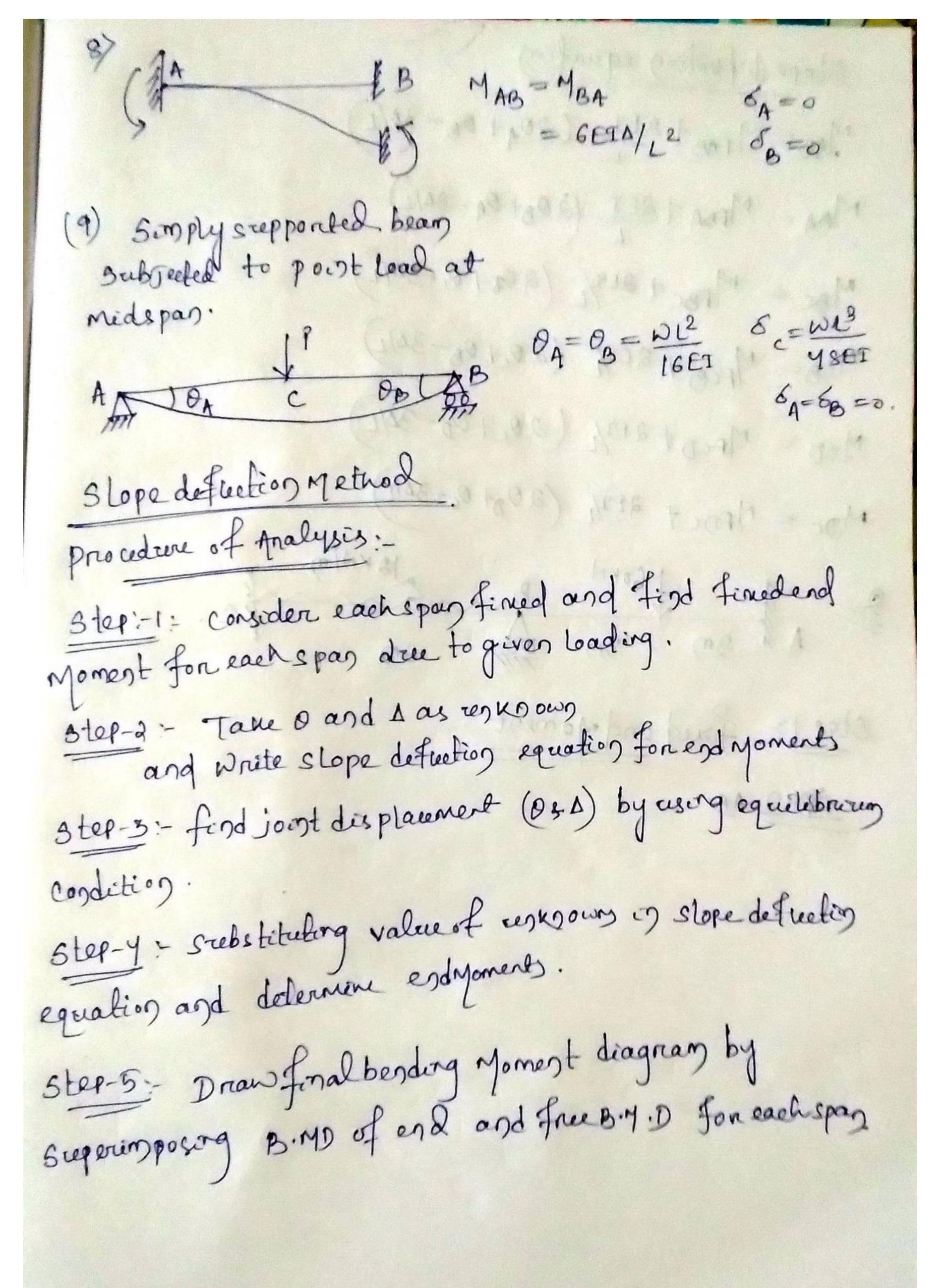
Stope de fuotion equation MAB = MFAB + 2ET (204+ 00-30/L) MBA = MFBA + REI (20B+ DA - 8A/L) MBC = MFBC + 2ET/L (208+0c-30/L) MCB= MFCB+2E9/2 (20c+0B-34/4) MCD = MFCD + 2 ET/L (20c+00-3AL) MDC = MFDC+ 2ET/L (200+0c-34/L) 2 1 GOKH BUSIN 3m 60 6m Ster-1: fined end Moment = 1-60 X 6 = -45 KNm:
