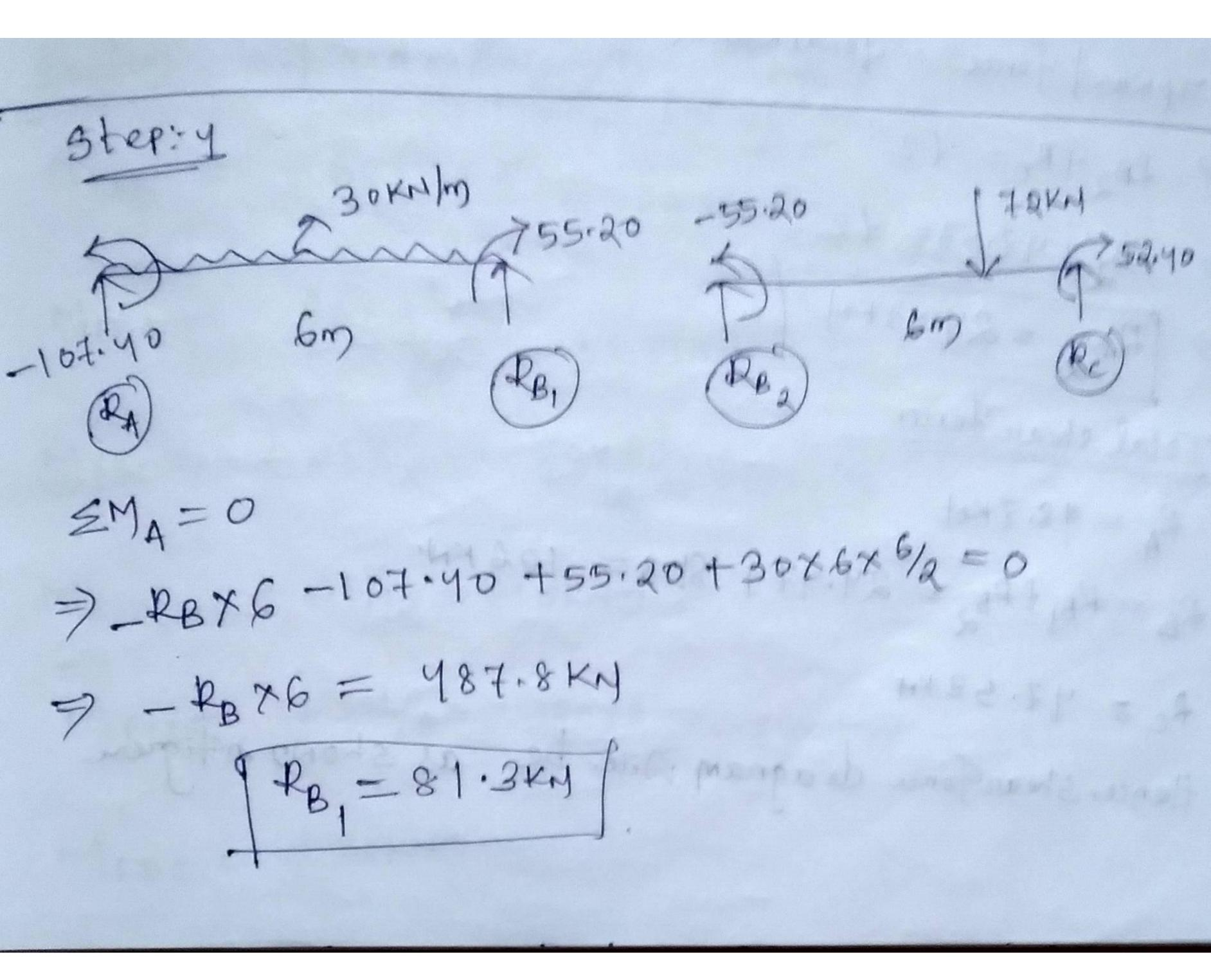
repward fonce = down ward fonce 7 RATRB = 30×6 > RA + 81.3 = 180 7 RA = 98.7 KM d'orebean BC: SMB-0 -Rcx6 -55-20 +52.40 +72x4=0 -Rexb = 285.2 Rc= 47.53KN repward fonce = down ward fonce > 2B2 + Re= +2 > RB2 +47.53= 72 => RB2 = 24.47 KM Total shear force RA = 98.7KM RB = RB, FPB2 = 24.47+ 81.3= 106 KN. RC = 47.53 KM Hence skearforme déagram will be as shown infigure
